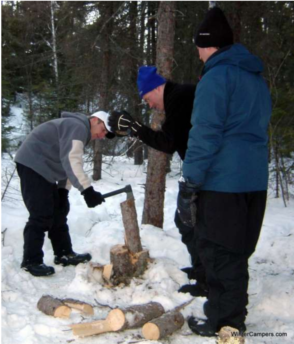
A SAFE SETUP FOR SPLITTING WOOD: PAUL KEEPS THE HATCHET HEAD SECURE IN THE BLOCK, MARK HAMMERS THE HATCHET HEAD WITH A WOODEN BLOCK AND JASON CLEARS AWAY SPLIT BLOCKS.
